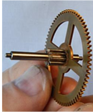
Figure 85 – intermediate wheel and pinion
