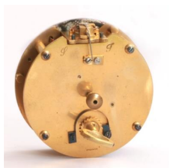
Figure 20 – drum movement showing platform escapement
