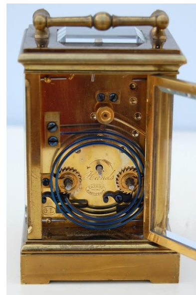
Figure 17 – carriage clock rear, showing attractive finish
