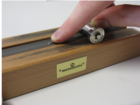
Figure 109 – using a screwdriver sharpening device
