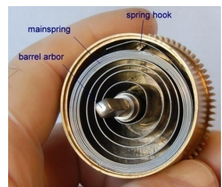
Figure 84 – barrel with end cap removed
