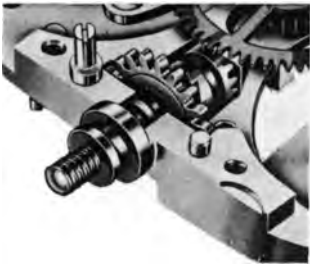
Plate V: Crown wheel and castle wheel.
