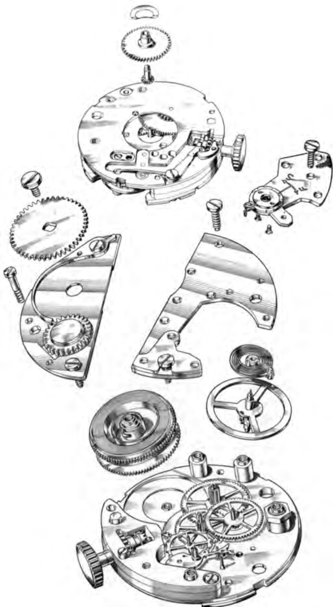
Fig. 22. Exploded view of general construction of inexpensive men's wrist-watch movement.
