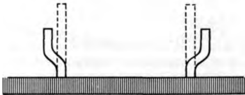
Fig. 42. Adjusting banking pins.
