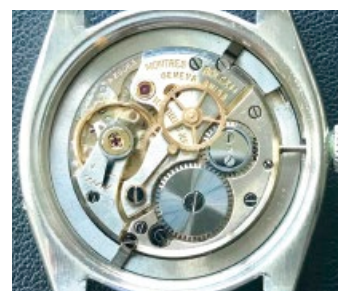
Caliber 1215 with unevenly aged service components (ratchet & crown wheels). The regulator is set to the minimum position, suggesting the movement is running fast and may be ready for a service.
