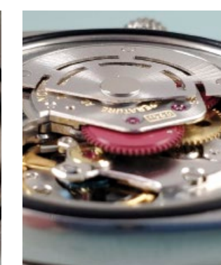
Caliber 1560 Movement in case | Reverser wheels | Autowind removed
