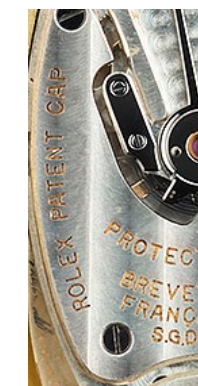
Vertical Geneva Stripes, Anglage bevels and screw sinks
