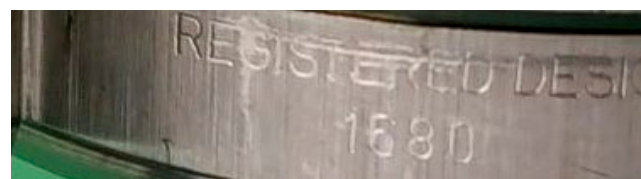
The brushed finish (vertical stripes) are a distinguishing characteristic of the way Oyster cases are made and can be challenging to fake
