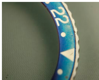
The blue pigment deteriorating to reveal the underlying silver color
