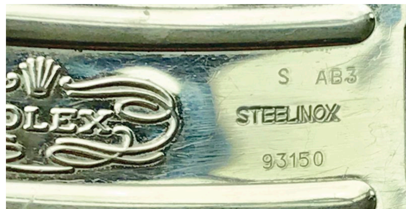
This is a Service Replacement clasp denoted by the 'S'. The AB3 code suggests production in the third quarter of the year 2000. The 93150 denotes an Oysterlock clasp for a Submariner or Sea-Dweller and should be paired with a matching Oyster bracelet marked 93150.
