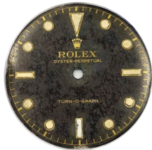
Aged tritium on a vintage Turn-O-Graph circa 1950s. Note the cream hour markers and the inconsistent 6 o'clock marker. Overall originality is inconclusive but most likely a vintage-relume.
