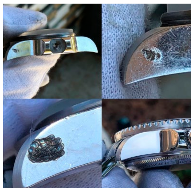
Benchtop laser welding has been common practice in the jewellery industry. Similar techniques are being widely used in vintage watch restoration and case repair.
