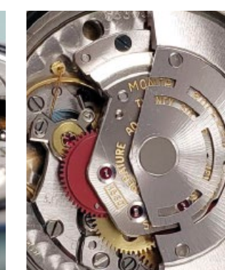
Caliber 1560 Movement in case | Reverser wheels | Autowind removed
