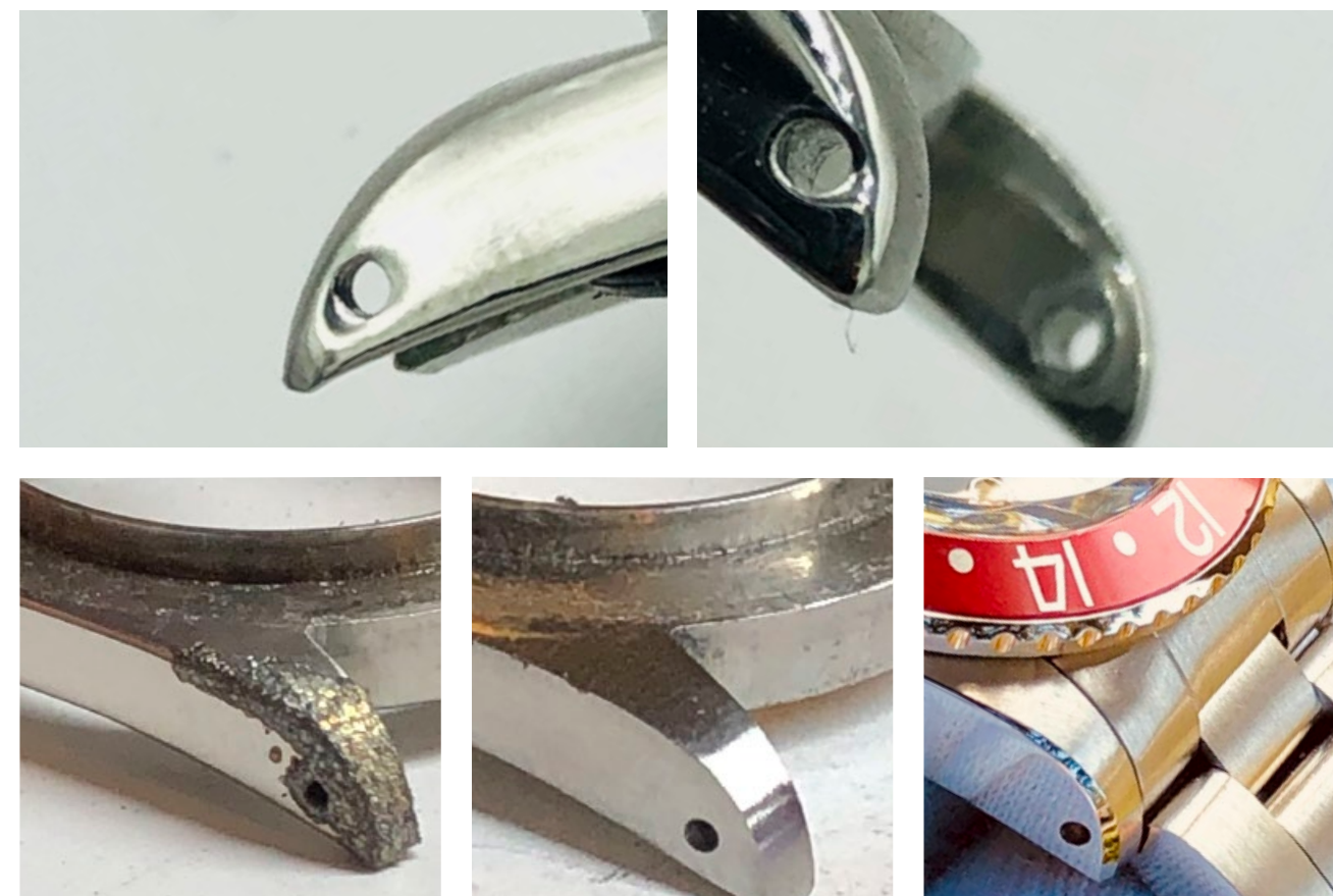
Top: Over-polished damaged lugs. Excellent candidates for restoration through laser welding and milling. Bottom: After laser welding, then recut (milled) with a chamfer.
