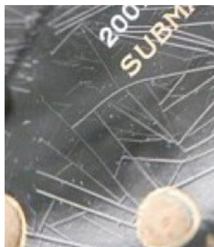
Lacquer defects can result in eventual cracking, giving rise to the creatively-named spider dials. If uniform and symmetrical they can be attractive but the long-term prognosis is not good. If left untreated and stabilized the lacquer will eventually chip and flake. Caught by moving hands it will scratch the dial leaving drag marks, before being ground down and making its way into the movement.
