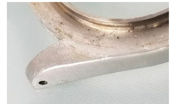
Early stages of pitting commonly appear on the top of the mid-case beneath the bezel ring. This is a challenging area to clean without disassembling the case.
