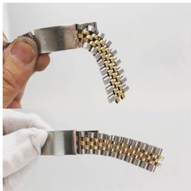
Bracelet stretch (before) and restoration (after). While bracelets are considered consumable and replaceable parts, they can be restored and reconditioned, complete with exotic finishes (courtesy Rolliworks)
