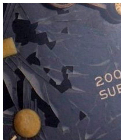
Lacquer defects can result in eventual cracking, giving rise to the creatively-named spider dials. If uniform and symmetrical they can be attractive but the long-term prognosis is not good. If left untreated and stabilized the lacquer will eventually chip and flake. Caught by moving hands it will scratch the dial leaving drag marks, before being ground down and making its way into the movement.
