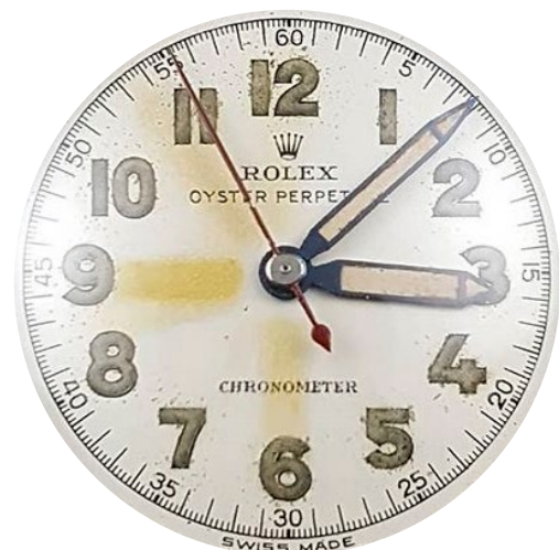
Radium burn on a vintage Bubbleback 2940 circa 1940s. The lume has assumed a distinctive olive green hue.
