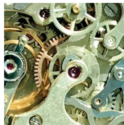
A generic Valjoux 23 in a Rolex ref. 2511 mid-size chronograph. It is a generic donor movement making this watch a Franken at best, and an outright counterfeit at worst.
