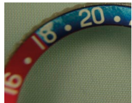
The blue pigment deteriorating to reveal the underlying silver color
