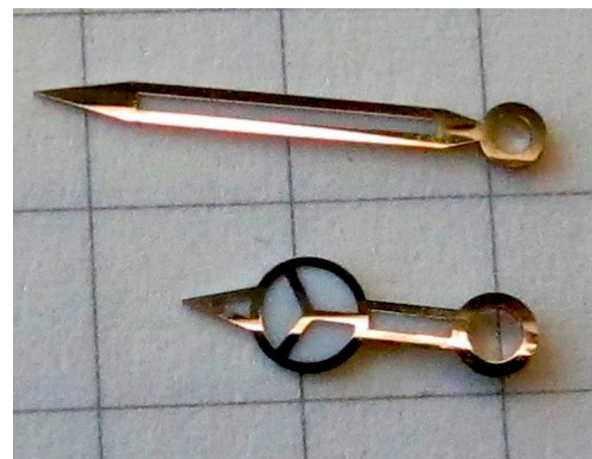
Contemporary and Service hands have a curved (convex) profile which reflects light differently from flat vintage hands. This example is filled with bright white Luminova which is the first indicator of age. You may encounter curved, modern hands that have been relumed with aged tritium.
