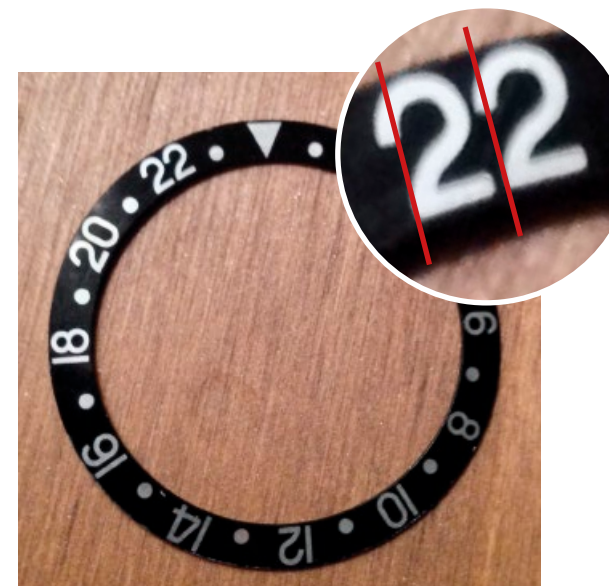
A very common fake bezel known as the “hooked-two”, for a GMT-Master II reference 16710. The hook of the “2” extends beyond the horizontal base leg
