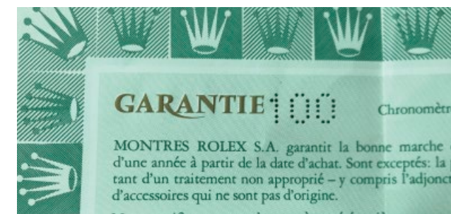
Warranty paper punched numbers are 4 x 6 holes. Counterfeit papers are sometimes punched with 5 x 7 or 5 x 9 holes.
