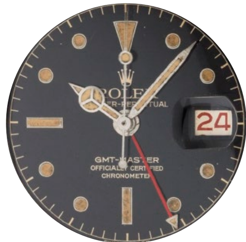
A typical moisture-damaged tritium dial and hands from a GMT-Master 1675 circa 1960s. Note the almost moldy appearance of the lume.
