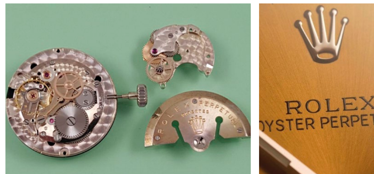
Movement (left), auto-wind assembly (right top) and semi-circular rotor weight (bottom right)
