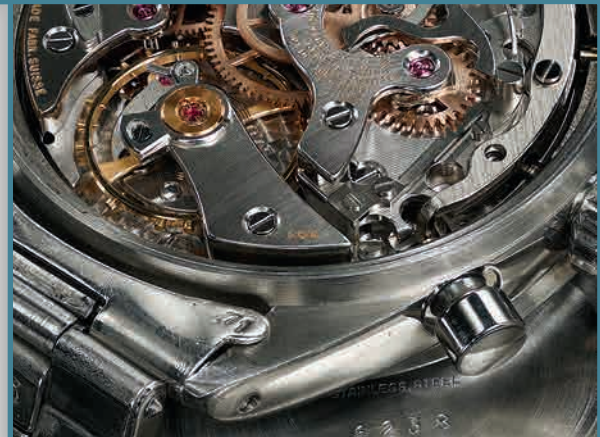
DETAIL OF THE CLOVER-SHAPED KIF SHOCK ABSORBER AND ROW STAMP - ENLARGED SHOT OF THE DIAL WITH UNDERLINED GRAPHICS - ANGLED IMAGE OF CASE PROFILE, BEZEL, CROWN AND PUSHERS.
