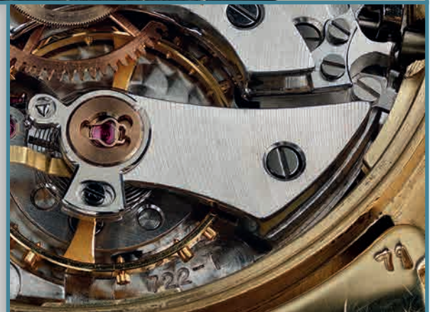
DETAILED SHOT OF THE MOVEMENT SHOWING THE SHOCK ABSORBER - MAGNIFIED DIAL IMAGE SHOWING REGISTERS, CROWN LOGO AND GRAPHICS - CASE BACK RETAINING FACTORY STICKER.
