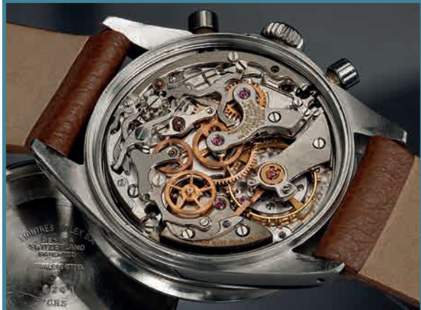
INSIDE THE MOVEMENT AND REAR VIEW OF THE CASE BEARING PUNCHED MARKS - ENLARGED PHOTO OF THE CROWN LOGO AND GRAPHICS - SHOT OF THE CASE PROFILE WITH CROWN AND PUSHERS.
