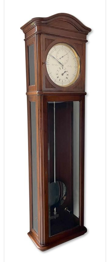
An Austrian precision regulator with a later Riefler K pendulum, No. 4254, DRP 100870
