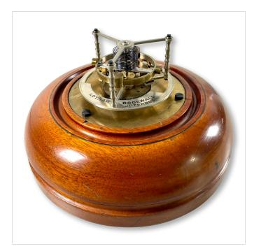
A rare escapement model with flying tourbillon regulator and pivoted detent escapement, made in Jüterbog by a student of the German Watchmaking School Glashuette
