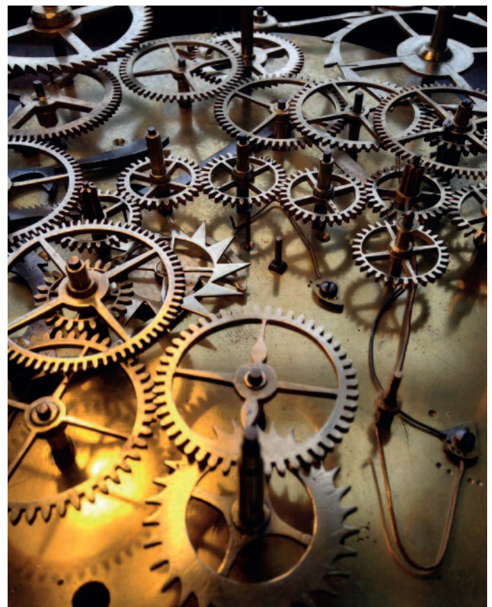
A complicated striking regulator with calendar and moonphase by Thomas Morgan of Manchester, c1860 – the type of complicated clock that Adrian most enjoys working on.
