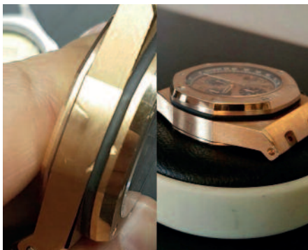
A damaged Audemar Piguet 18K rose gold watch – and after being filled and valeted back to satin finish.
