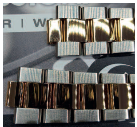
The top picture shows a Rolex submariner bracelet with a large dent in the centre link which is hollow 18 carat gold. Below is the link filled with gold and then re-finished, rather than the dent being simply polished out.
