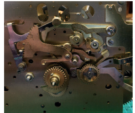
A different version of a chain wound clock showing auto night shut off.
