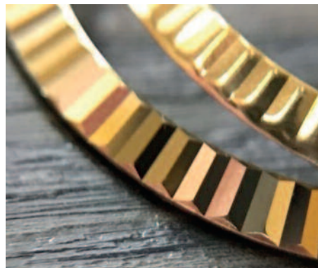
Before and after effects of re-cutting a fluted bezel. Rolex do not provide this service.
