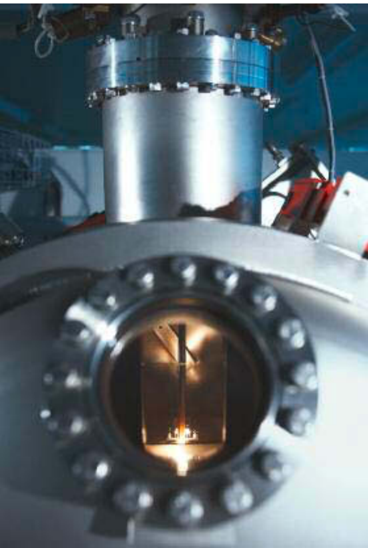
The Parachrom is made in a giant furnace (above, left) with a porthole (left) for viewing the alloying process (above).
