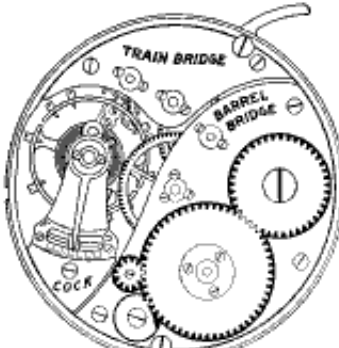
Hunting, Lever Setting with Winding Indicator
