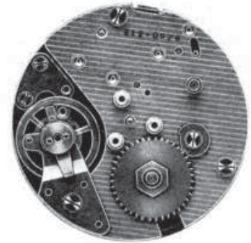
Movement with pin lever escapement Diameter 44,8 mm. 1 day (40 hours) Alarm Key winding
