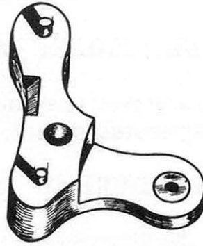
Chronograph Pivoted Detent Bridge Assembly 42
