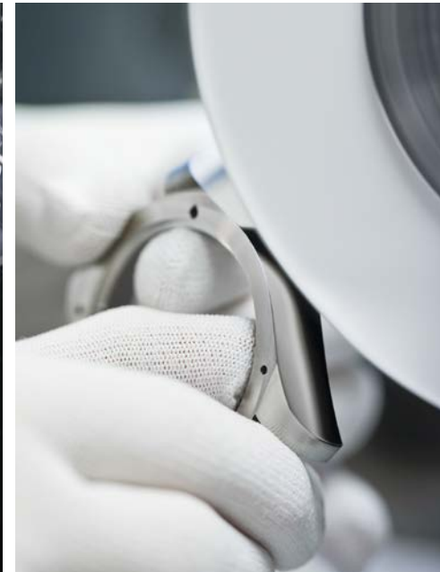
Left: a 904L steel blank for the watch cases is ready for machining.
