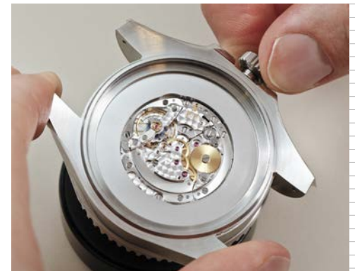
Specialist watchmakers dealt with the highly sensitive task of assembling each watch. From top to bottom: the dial is placed on the movement. The centre hands are placed on the dial. The movement and dial assembly are placed in the middle case. The winding crown is fitted.
