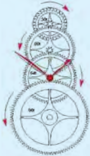
Figure 4: This is an accurate drawing of the proportions of the direct drive movement being designed on these pages, but it is not yet dimensioned since the actual size of the wheels and pinions (as opposed to the count) has not been decided. The only things that need to be done to make this a working drawing for the train is to determine the gear tooth size (the module), pivot, and mounting details.
