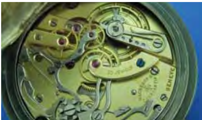
Figure 1: Movement of the Vacheron & Constantin chronograph railroad watch
