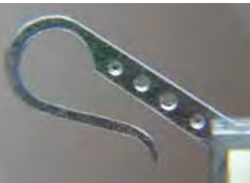
Figure 4: Filing to the correct size and shape
