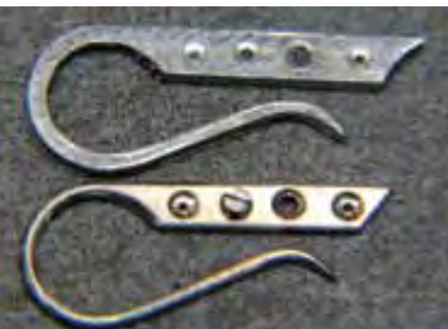
Figure 5: Beveling and flat polishing for the swan neck
