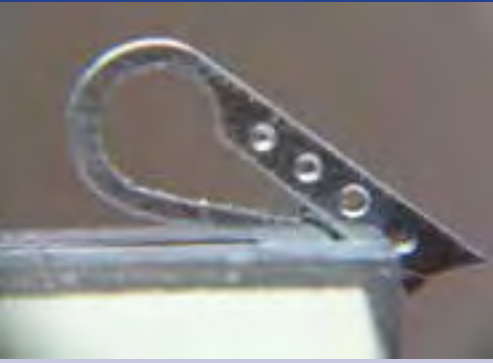
Figure 3: The piece after sawing extremely close to the trace lines
