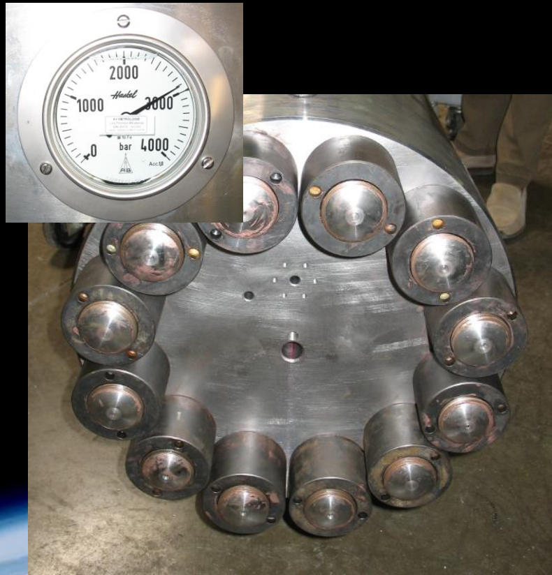
Development of a temperature controlled testing chamber for 3000bar
