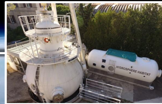
Hydrosphere hyperbaric and hypobaric tests. The facility includes a habitat for tests with humans.
