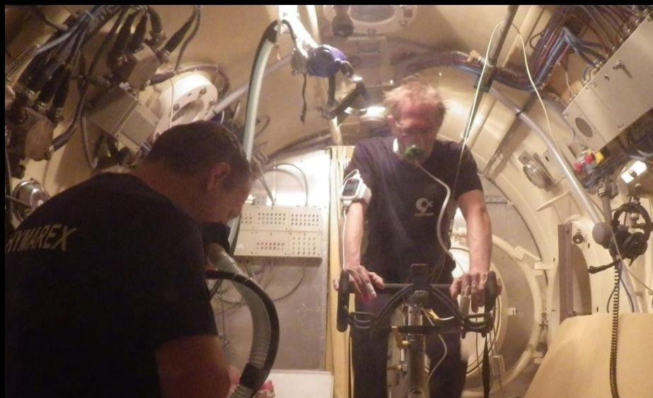
High-altitude tests with a COMEX' subject in the low pressure chamber (Photo: L. Negrel, COMEX)
