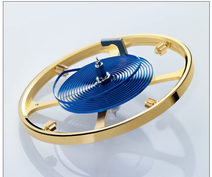
Figure 5. The balance assembly from the 32- family of calibres is fitted with a 'Parachrom' balance spring, which contains a high proportion of niobium and is said to be paramagnetic.
